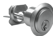
CBR114-SCKD 6-pin, brass rim cylinder with aluminum clad face. 1¼" (32 mm) long with 2⅞" (62 mm) tailpiece. Schlage keyway.
