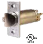
DGPL238 Deadlatch: 2 3 / 8 " (60 mm) backset, 1 1 / 8 x 2 1 / 4 " (28.5 x 57 mm) faceplate
