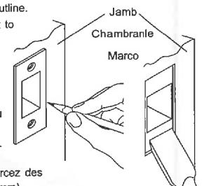
**I.** Place strike box in jamb, align strike over strike box and trace outline. Chisel out area traced, deep enough to allow strike and strike box to install flush with jamb. Place strike box and strike in jamb and mark screw hole centers. Where marked, drill 3/32" diameter pilot holes, 1" (25mm) deep.
