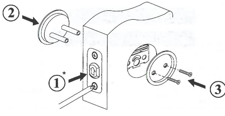
\*Proper installation allows the "thumb pull" to open from bottom, as shown.
