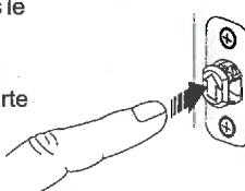
To operate thumb pull, depress to extend, depress to retract. Keep the thumb pull retracted after use.
